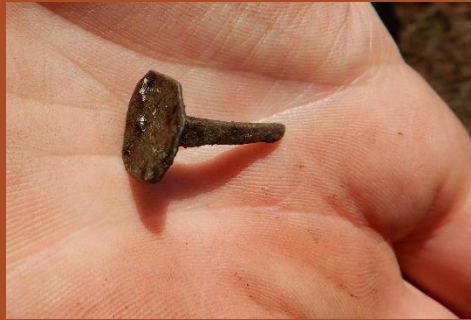
Hand-forged copper nail
